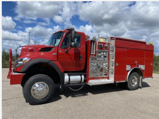
Salvaged commercial boom truck “Reconstructed” into Fire Truck.
