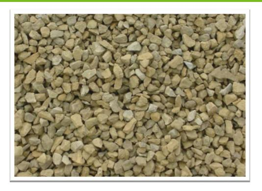
• Crushed stone- A product of mechanically breaking down bedrock.
